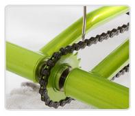
Apply a moderate amount of oil along the chain. Release the brake, and raise the left rear drive wheel off the ground and rotate the pedals to distribute the oil evenly.
