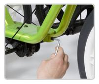
Use the 3/16" hex-head wrench to tighten the cap screws at the front of the plate. This tightens the chain. When the chain tension is right, tighten the 2 cap screws on the top of the crankcase. (If the chain tension is fine to begin with, it is still a good idea to check the tightness of the 2 cap screws).
