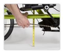
To check the chain tension, lift the lower chain. There should be no more than 1" of deflection.
